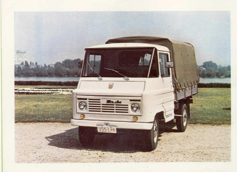
ŻUK A11B Delivery Van is destined for transportation of cargo up to 1100 kg.
