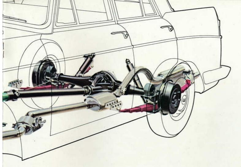
The 2912 c.c. six-cylinder engine transmits power via a diaphragm spring clutch with hydraulic actuation to a four-speed gearbox with centrally mounted gear lever. The exhaust system is flexibly hung at all points and, together with rubber mountings for power unit and suspension, ensures maximum insulation against sound and vibration.
