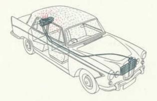
NORMALAIR Air Conditioning is available on the Wolseley 6/110 Mk. II as an optional extra. The system, which incorporates a refrigeration unit, is a boon in hot or humid climates, allowing the gentle circulation of cool air without the inconvenience of wind noise from open windows.
