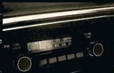
AM/FM 5 push button radio with three speakers (auto-search radio/8 track stereo on Special).
