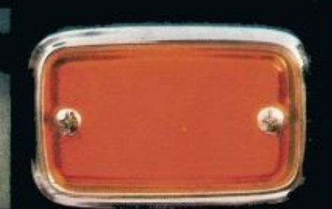
Red safety light on rear passenger doors when open.
