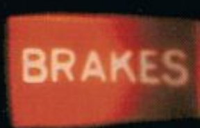
Brake fluid level warning light.
