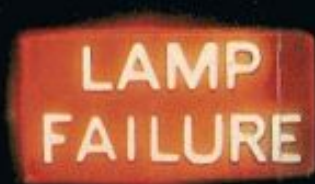
Stop and tail lamp failure warning light.
