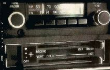
Three speed heater/demister with illuminated controls (Air-conditioning on Special).
