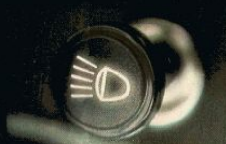
Light switch and rheostat panel light control.
