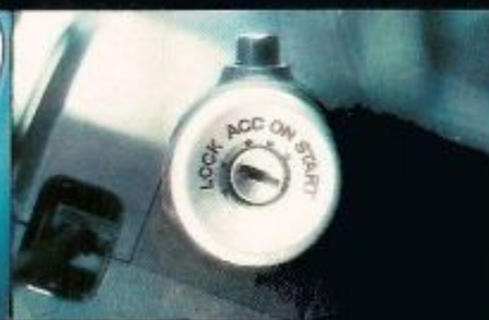
Steering column lock with alarm (open door with key left in and alarm buzzes).
