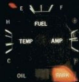
Low fuel indicator light. Handbrake warning light.
