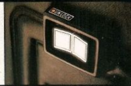
Electro magnetic door locks—all doors lockable from drivers position.
