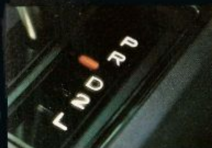
Toyoglide three-speed automatic transmission with T-shift (column shift on Estate).
