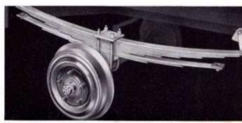
Long, flexible, easy-riding, two-stage rear springs are standard. Big, powerful, dependable, self-equalizing hydraulic brakes of latest two-shoe type give your Coupe Express the surest of stopping ability. Parking brake is on rear wheels, independent of load. Composite brake drums assure long lining life, cool operation, and freedom from warping and scoring. Proper load balance further enhances roadability.
