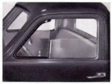
Perfect ventilation in any weather. Vertical metal division moulding lowers with window glass, affording free arm-room for signaling. Angle-set vanes may be kept open in driving rain — an exclusive feature. Comfortable in summer and winter alike.
