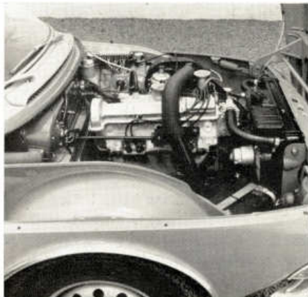
The modern four-cylinder engine has an overhead camshaft and is mounted together with the transmission into one compact unit.
