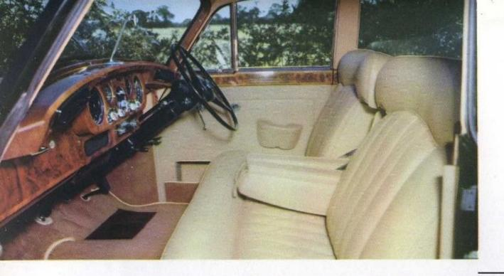
Driver and passenger can adjust the rake of the front seat independently. Elbow rests on the doors are adjustable and the centre armrests fold away if a third person is carried in front. Also visible in this view is the ride control switch on the steering column. A picnic tray and ashtray pull out from under the fascia panel.
