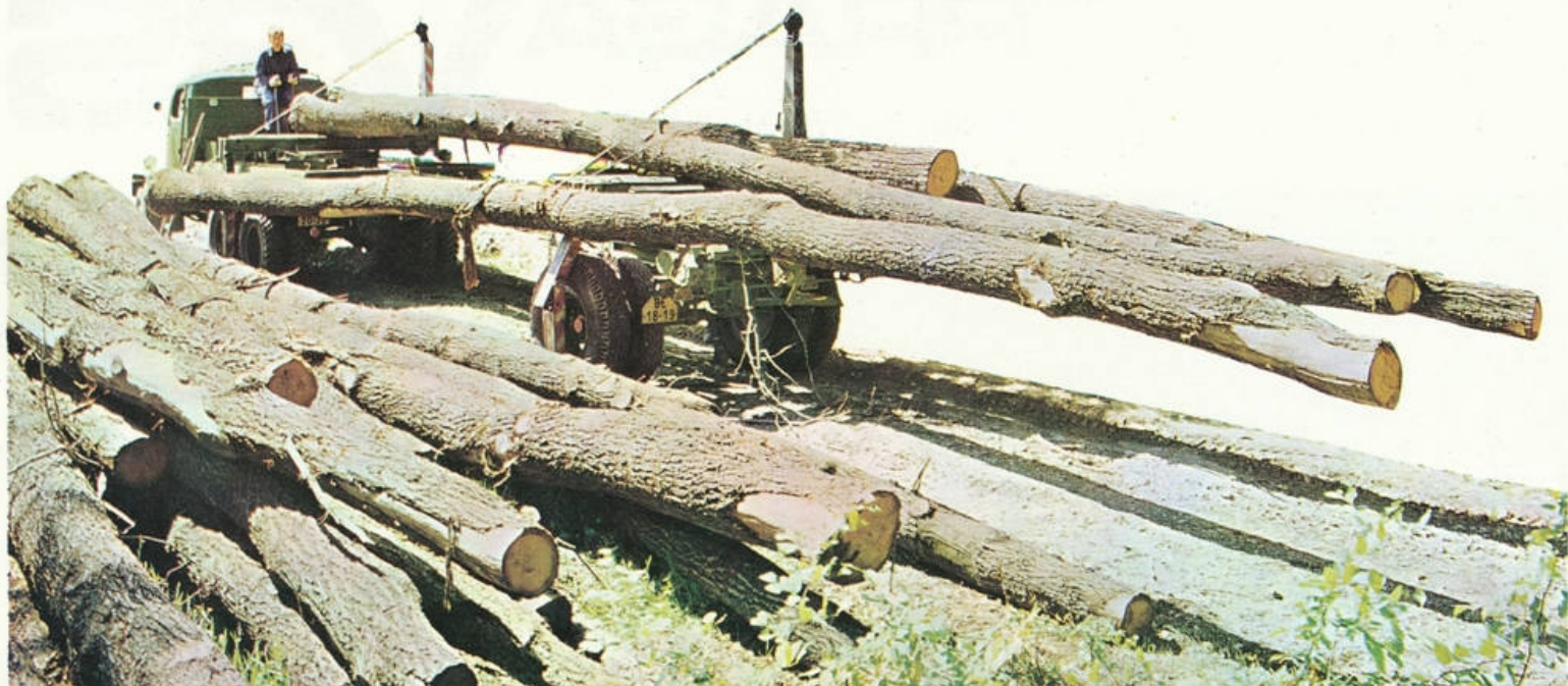
Quick and fully safe cross-hauling and stacking of log timber by means of trailer tractor double-drum power winch.
