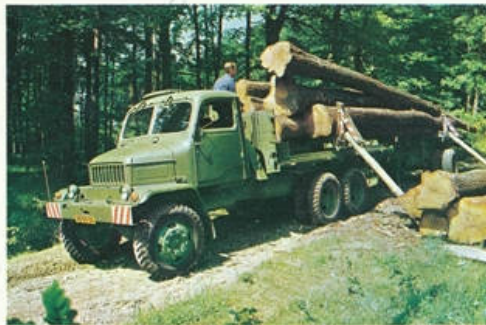
Quick and fully safe cross-hauling and stacking of log timber by means of trailer tractor double-drum power winch.
