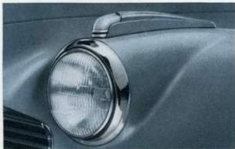
New Sealed Beam headlamps with separate parking lights are moulded into contours of the fenders.
