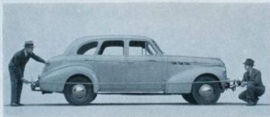
Over-all length is greater on all 1940 models. Pontiac wheel-bases range from 117 inches to 122 inches in three steps.
