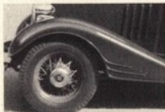
This fender design prevents road splash and cuts down the frequency of car washings.
