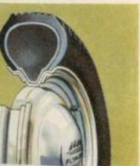
Safety Rim Wheels hold tires in position on rim in case of blowouts, insure safer stopping.
