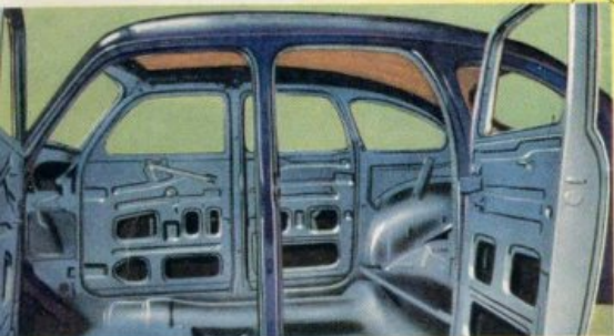
Steel Body gives the new Plymouth great strength. The steel floor, front and rear crossmembers, steel side-panels and one-piece steel top are all welded into one solid, rigid, safe unit. The new Plymouth is built for rugged duty.
