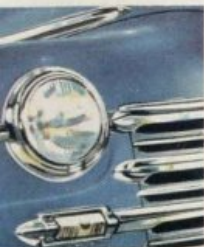
Dual-Beam Headlights provide maximum lighting. High beams are foot controlled.
