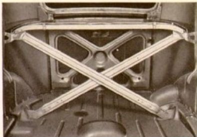
This massive X-brace in the rear of sedans having built-in trunks provides unusual reinforcement.
