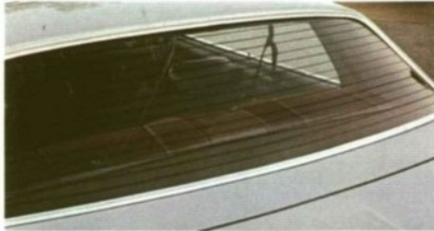
Electric Rear Window Defroster clears window quickly with heating elements fused to the glass.
