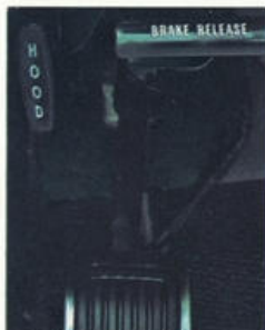
Inside Hood Release. It protects against the hood being opened from the outside.
