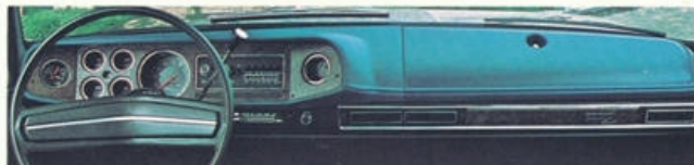
New Instrument Panel. Features tach, clock, oil, amp and temperature gauges.
