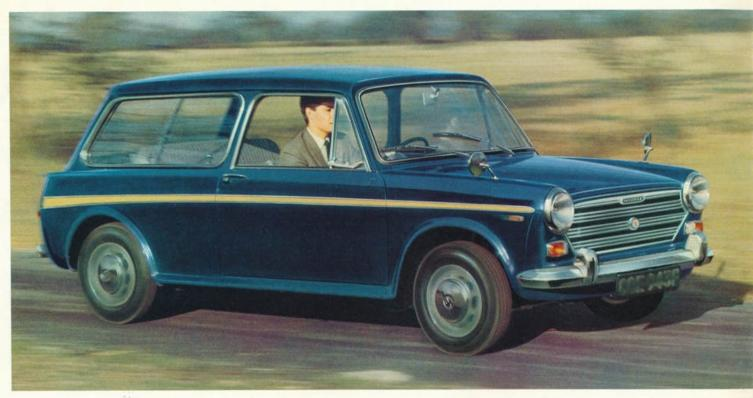
Quick and easy loading even with hard-to-handle cargo. The full-width rear door swings high out of the way. Counterbalancing makes it light to handle and a safety device holds it firmly open. Light enough for a woman to open and shut one-handed with no effort at all. The total loading capacity is 37-7 cu. ft. and the loading at the rear of the back seat is 14 cu. ft.
