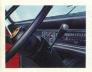
This is the fascia fitted to all 1300 two- and four-door Super De-luxe Saloons. All the instruments are grouped on an easy-to-read panel. A new, all-in-one switch on the steering-column controls dipswitch, horn, indicator switch, and headlamp flasher. And the glove compartment and wide parcel shelf accommodate a vast amount of odds and ends.
