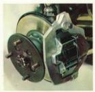
Powerful brakes (single calliper disc at front) make these new Morris cars some of the safest on the road. The extra power of this brake is also provided on 1100 Mk. Il cars when fitted with automatic transmission.
