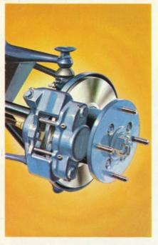
'Safety Fast' is not only a slogan as far as M.G. are concerned—it is also a principle. That is why the M.G. 1100 is fitted with powerful hydraulic brakes—8" discs at the front and 8" drums at the rear. A pressure limiting valve is introduced between the master cylinder and the rear drum brakes to more accurately apportion braking between front and rear wheels for both wet and dry road conditions.
