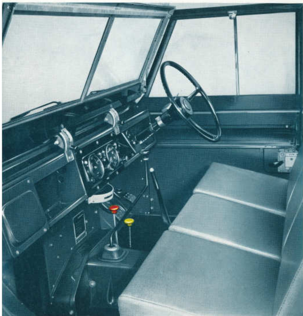
Cab for diesel models shown. Hand throttle control extra on petrol models.
