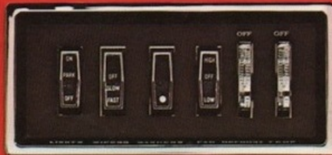
Instrument control panel has individual recessed switches.
