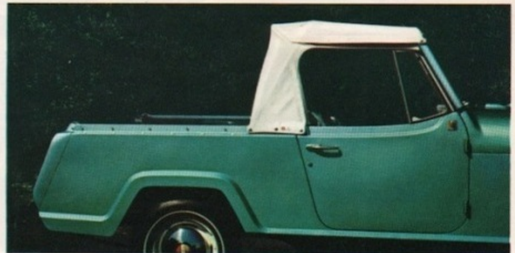
Half fabric top provides pick-up truck function. Standard metal doors offer protection to passenger and driver . . . roll-down side windows are glass.
