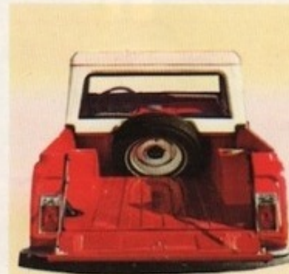
Spare tire is mounted to allow full use of cargo area, yet permit driver's unobstructed view through rear window.
