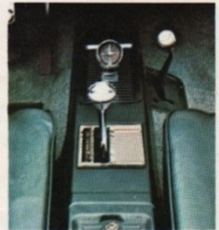
Sporty console with map case and gear box available on some models. Single-lever 4-WD control is standard.
