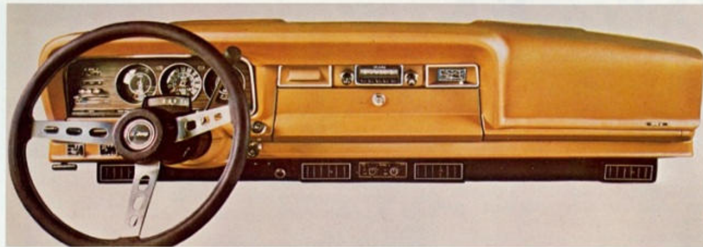
Instrument panel with optional air conditioning, "Soft Feel" sports steering wheel, AM/FM stereo radio, electric clock
