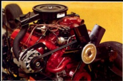
Power-packed V-8. A 345 cubic incher that delivers all the power you'll ever want. Meets all emission requirements. Available with automatic choke, and modulated fan to save gas.
