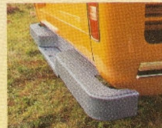
Heavy-duty step bumper. It makes it nice and easy to load up the bed and tow up to 2000 lbs.
