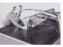
New color-keyed tonneau cover snaps on neatly and quickly. Protects driver and passenger compartment from dust, dirt and rain. Converts from one piece to two pieces in seconds. Simply unzip it and you can remove cover from driver's side.
