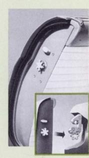
New Lifeguard door latches have a new double-grip engagement to help keep doors from springing open . . . give added protection against occupants being thrown from the car should an accident occur.
