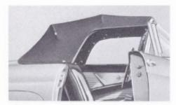
This year, color harmonies start with the roof and run clear through to the steering wheel. The smart, new black rayon convertible top, above, folds right down out of sight behind the seat. A white, fabric-grained vinyl top is also available.
