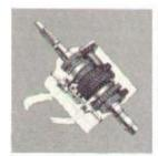
SYNCHRONIZED TRANSMISSION Brand new for '63 and only Ford has it! For the first time, low gear is synchronized as well as second and high. Now you can downshift into low without clashing gears while still moving forward . . . main-tain momentum. Saves
