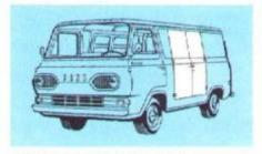
NEW LEFT-SIDE CARGO DOORS. To provide you with even greater flexibility and ease in leading or unloading, a left-side double cargo door is available on '63 Econoline vans.
