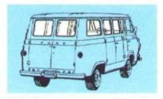
DISPLAY VAN. The display van has windows in the right side of the cargo area. This provides good lighting for bins, etc., custom-built against the left wall. Rear windows optional.
