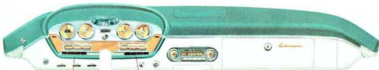
CONTROL CENTER INSTRUMENT PANEL. —Following advanced aircraft practice, the Edsel panel places instruments, control
