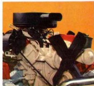
New V-8 Engines —with bigger 361 cu. in. displacement, higher 10 to 1 compression ratio, increased torque, greater economy.
