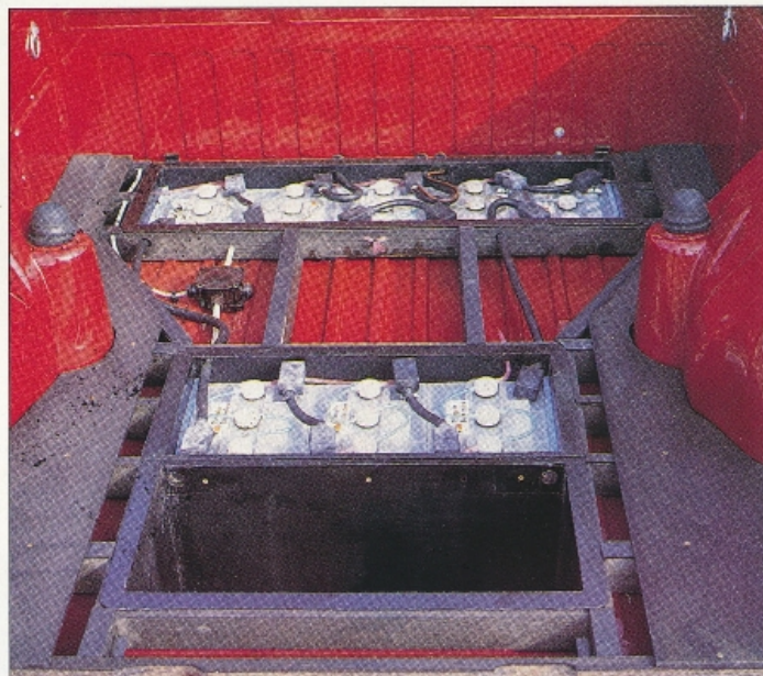
Storage batteries in the rear section of the electric vehicle
