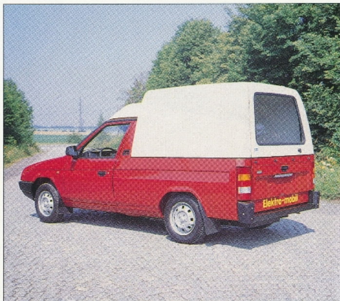
Pick-Up Electro with storage compartment hood made of composite plastic
