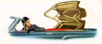
AUTOMATIC TOP It is an old Chrysler feature, but it is a great concenience - the automatic, electrically operated top. Merely turn the lever, and the top folds up or down in the matter of a few seconds. New this year is the top "hangar" that is flexible and can be pushed out of the way, making more room in the rear deck compartment.
