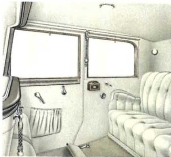
A full disappearing glass partition separates the driving compartment from the tonneau. This model can be either Sedan or Limousine at will
