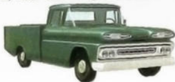
CHASSIS-CAB MODEL C1403 —Special utility body mounted on a 115" wheelbase chassis-cab demonstrates versatility; and 5,200-lb. maximum GVW allows for plenty of heavy equipment.
