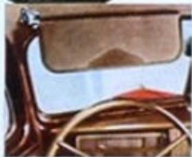
The sun visor is adjustable. It can be swung to the side to cut off glare at the window.
