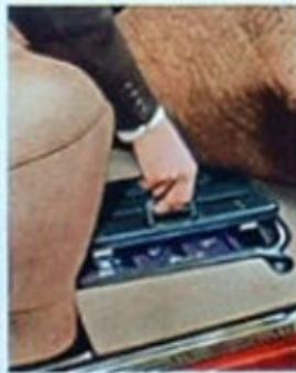
A snap-on rubber-sealed metal cover-plate makes the battery quickly accessible.
