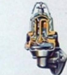
Air-pressure chambers in the fuel pump maintain a smooth flow of gasoline.
