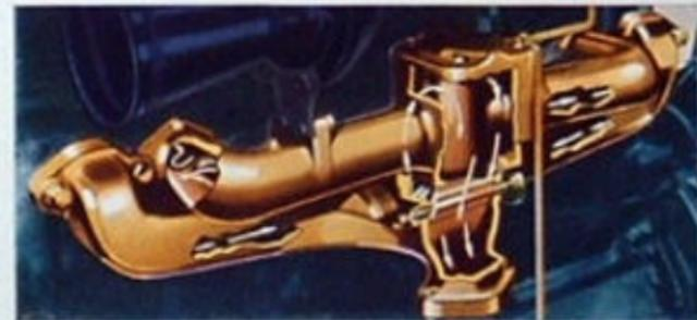
The temperature of the fuel mixture is regulated by a manifold warming-chamber with automatic thermostatic control.
