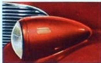
Slender headlamps are mounted on the fenders in fixed position.
