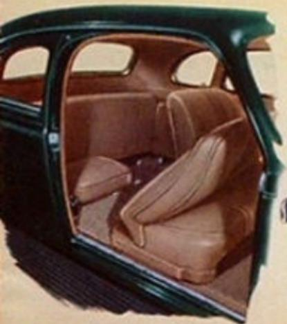
*The Four-Passenger Coupe has two interior seats in the rear of the passenger compartment. They fold up, out of the way, to make space for extra luggage.*
