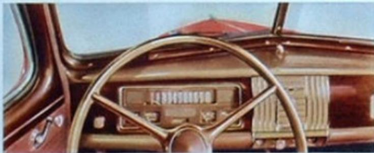
Clear-vision dials and accessible controls feature the instrument panel. Two defroster slots are provided for use when a car heater is installed as extra equipment. (Master De Luxe panel shown.)
