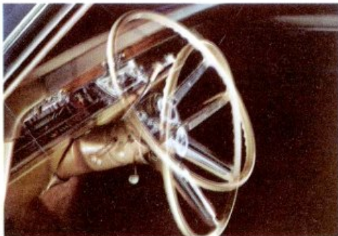
Comfortilt Steering Wheel —Adjusts to any of seven positions to accommodate tall or short drivers. Wheel can be raised out of the way for easier exit.
