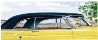
The Convertible top for 1953 is offered in four different shades —black, tan, blue and green. Made of a durable, high-count rayon and cotton fabric, these tops are cushioned with an inner layer of rubber for additional insulation and waterproofing. Wide vision, unusual headroom and sound construction make the Cadillac Convertible an excellent year-round motor car.
