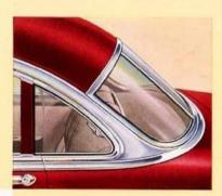
Rear and side vision is greatly improved by the new narrow rear quarter panel which because of its construction greatly increases structural strength. The wide clear-across curved rear window frame and corner pillar are in bright chrome.
