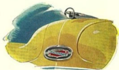
Beauty Feature with a Breezy Function—Smart note with a smart idea is the new Buick crest set in a generous opening on the nose of the hood—inrushing air helps cool the engine compartment.
