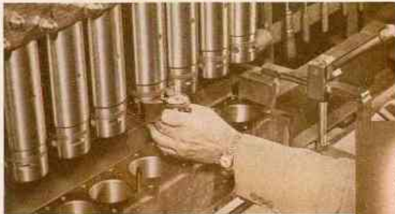
First bored with great accuracy, cylinders are then specially processed to provide an accurate "working fit" between piston and cylinders as though each were individually made for the other.
