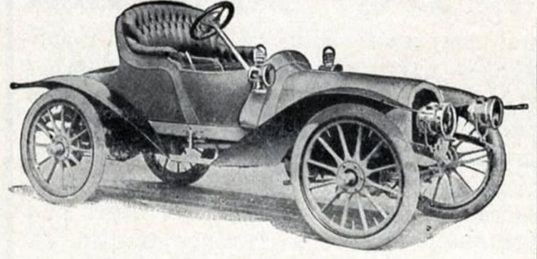
design of rare beauty. Different and superior to any other runabout. Graceful, fleetness in every line. Hard, dull oil-paint finish, wear-proof and scar-proof. Aeroplane Mud Guards—also entirely new—which lighten the car in running and make steering easy; no mud can reach body or occupant. 36-inch wheels. Silent running. 50 miles an hour. Air-cooled Motor, reliable every day of the year. A staunch, swell Touring Runabout, \$2,000 f.o.b. Detroit.
