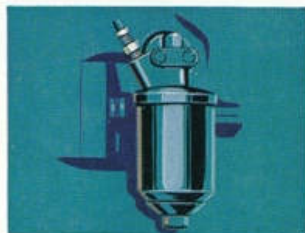
2. A full-flow oil filter is fitted externally, the element of which can be easily replaced.
