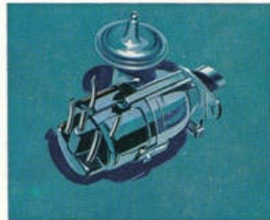
3. Ignition is by oil-filled coil, and distributor having automatic advance and retard assisted by vacuum control.
