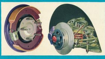
Large diameter hydraulic drum brakes are fitted on the rear wheels and with 11½ (0.29 m.) diameter disc brakes on the front wheels, are servoassisted to inspire confidence at the high speeds of which this car is capable. Sturdy, independent front suspension units and long rear semi-elliptic leaf springs are controlled and stabilised by hydraulic shock absorbers and anti-sway bars.
