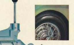
Basic models are fitted with ventilated steel disc wheels, but if continued high speed motoring, or excessive competition driving is intended, then wire-spoke wheels with "knock-on" hubs are strongly recommended. It is important that the choice should be made when ordering your car.
