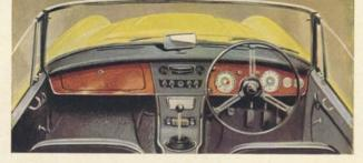
Essential for high-speed travel, the easily read instruments are closely grouped in a wood veneer panel in front of the driver. A short central gear lever in the console permits effortless changes and for driving comfort, the 17 inch diameter steering wheel has spring-spokes. A hard-wearing carpet over the entire floor completes the stylish interior trim.
