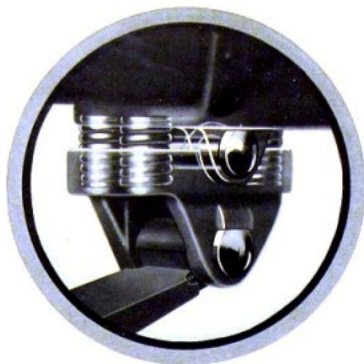
Four coiled springs encased at the rear of the left front spring accomplish magical results in steering safety and control
