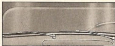
▲ WINDSHIELD WIPER for right-hand side of cab or driver's compartment; left-hand wiper standard.
