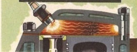
2-Way Gas Waste In Ordinary Combustion Chambers
