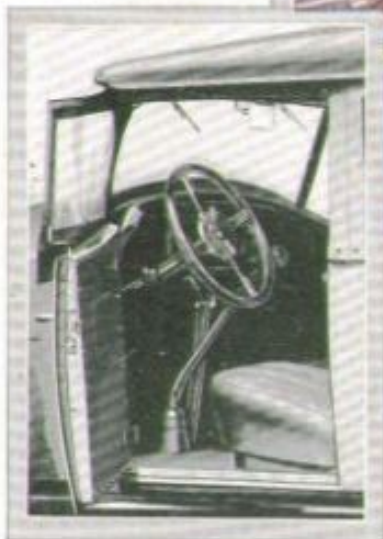
Side curtains, opening with the doors, are completely storm-proof and their extra large windows provide excellent driving vision in every direction
