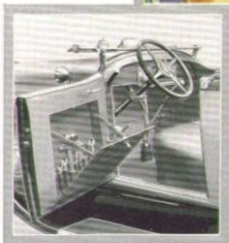
Here is the tool locker open, showing the convenient arrangement of tools. The view also shows the driving compartment, with instrument panel, steering wheel levers, and theft lock on the steering column
