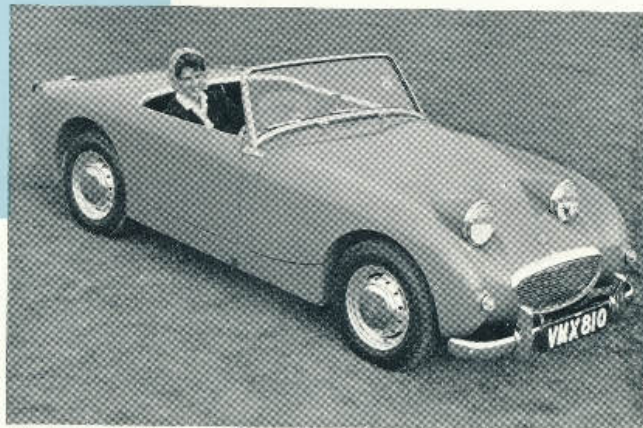
The first Austin Healey Sprites of 1958 had a one-piece, lift-up bonnet and front wings. Underneath was the famous 948 c.c. B.M.C. "A" Type engine which produced 42.5 b.h.p.
