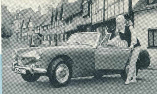
The Healey Sprite Mk. II, announced in June, 1961, had a restyled body with fixed front wings and headlights. The engine capacity was unchanged at 948 c.c. until the Mk. III Sprite came along with a 1,098 c.c. unit in 1964.
