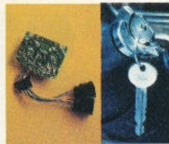
Solid-state ignition doesn't require breaker point replacement.
